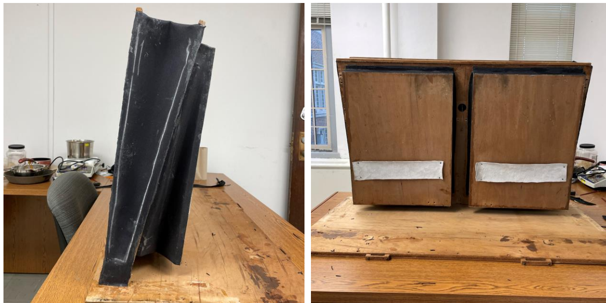
Figure 5. Two views of the bellows removed from the organ with the replacement rubber cloth. Left: Side view of the main bellows with the feeder bellows visible to the right side. Right: Front view of the two-feeder bellows attached to the main bellows. The leather strips cover a series of holes bored in the wood that serve as one-way valves, allowing air to flow out of the feeder bellows. Note: In these photographs, the bellows assembly is upside-down of its orientation in the organ. The proper orientation is depicted in Figure 4.
