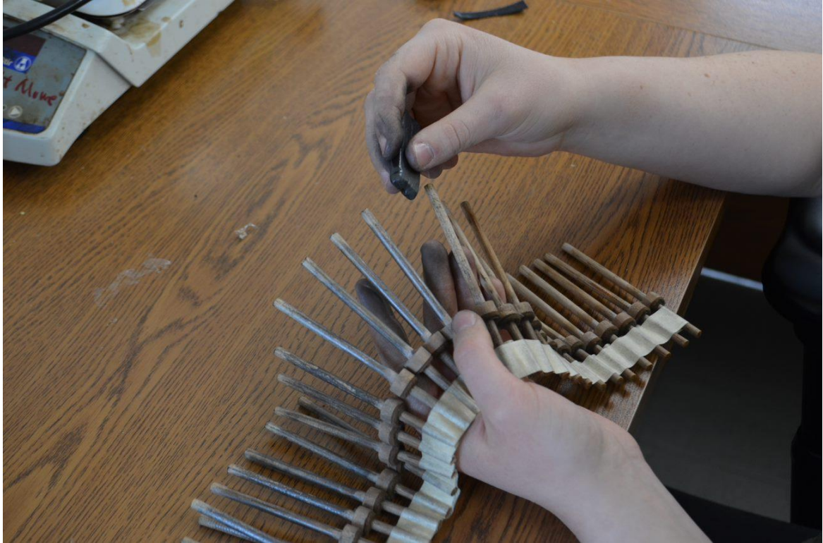
Figure A.6. Lubricating the stickers with crucible graphite.
