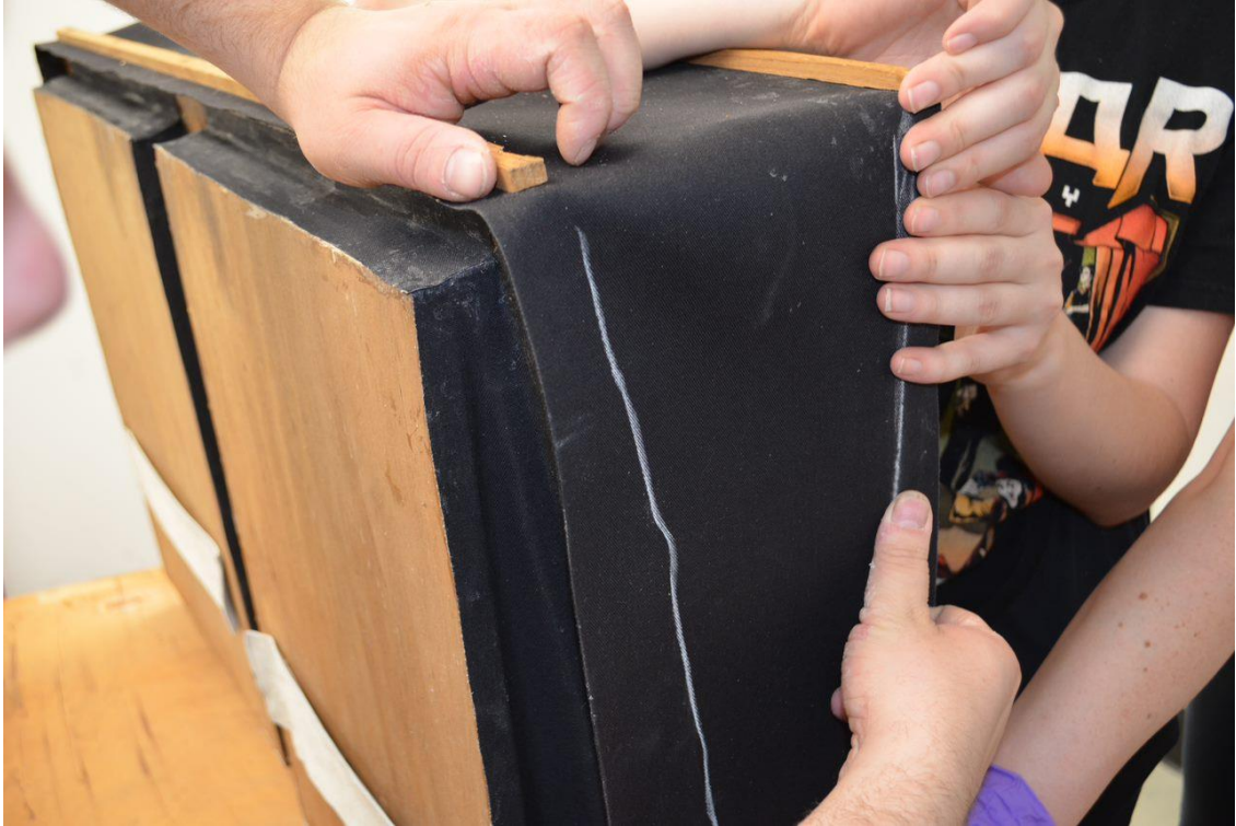
Figure A.4. Attaching replacement cloth to the main bellows.
