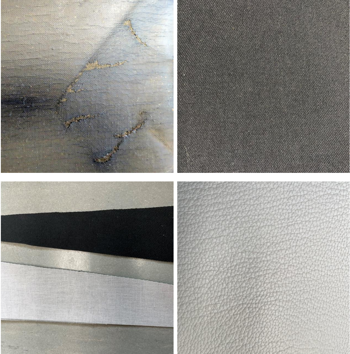
Figure 7. Original and replacement fabric components of the Beckwith reed organ. Top left: external side of the original rubber cloth for the main bellows. Deterioration of the cloth, where the rubber layer has been lost, revealing the fabric underneath, is visible. Top right: replacement rubber cloth for main bellows. Bottom left: replacement rubber cloth for feeder bellows; front side is black and back side is white. Bottom right: replacement leather.
