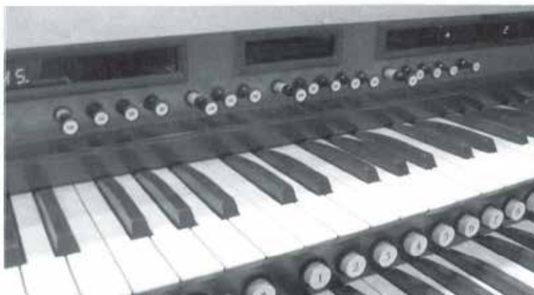
Six sets of expression shades, variable tremulants, and crescendo functions are assigned to five balanced pedals by these miniature drawknobs, which in turn are controlled by six independent combination thumb pistons.
